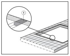
Grout lines ① and the hatched area underneath the surface of the appliance must be smooth and even. If they are not, the appliance will not sit flush with the worktop and the sealing strip underneath the top part of the appliance will not provide a good seal between the appliance and the worktop. All electrical work should be carried out by a suitably qualified and competent person in strict accordance with current local and national safety regulations (BS 7671 in the UK).
